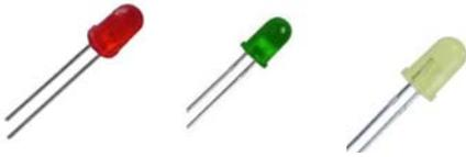
A range of 5mm diffused round LED's with an inbuilt IC to produce a continuous flash at a frequency of 3Hz. Supply voltage 9 to 12V. No series resistor required. Kingbright L-56 series.
